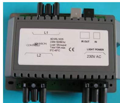
Figure 3: AD-IRL Integrated Lighting Control Module
