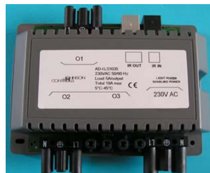
Figure 4: AD-IRS Integrated Sunblind Control Module
